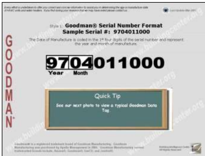
Figure 6 Example of Goodman serial number and determination of age of condenser.
